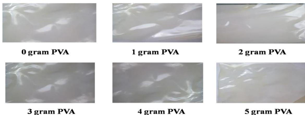
Figure 1. Tapioca-chitosan flour biofilm with variation of PVA
