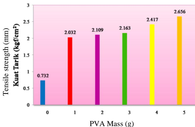
Figure 3. Effect of PVA mass on tensile strength of tapioca-chitosan flour biofilm
