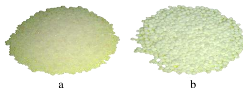
Figure 8. urea granules: (a) no coat, (b) coated
