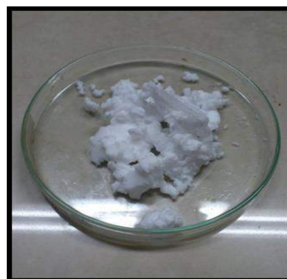
Figure 1. Crosslinked polymer deposits
