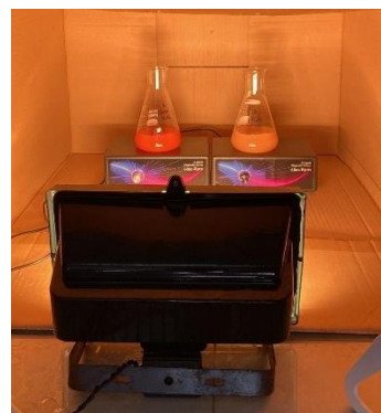
Figure 1. Batch system reactor design of methyl orange photocatalysis process
