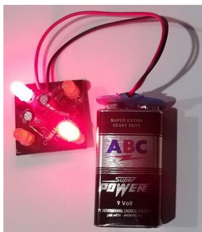
Figure 3. Assembled flip flop kit
