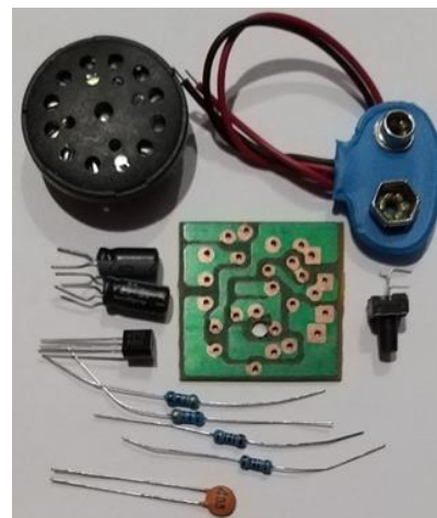
Figure 2. Components of a mini siren kit series
