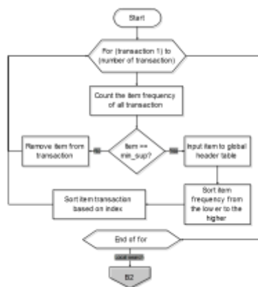
Figure 2. Flowchart of CT-PRO algorithm
