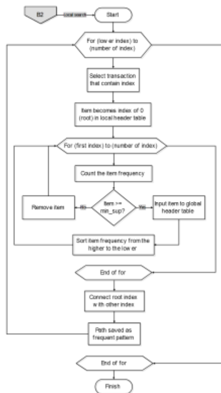
Figure 3. CT-PRO algorithm flow diagram (continued)
